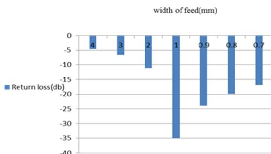
Figure 2: Variation of return loss with change in width of feed
