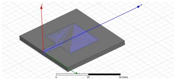
Figure 1: Structure of simple patch with line feed (units in mm)
