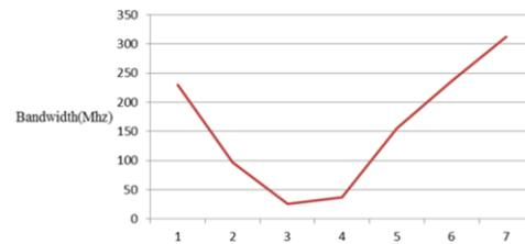
Figure 3: Variation of bandwidth with change in width of feed
