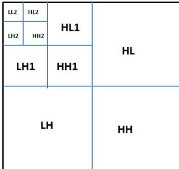
Fig.1: DWT decomposition
