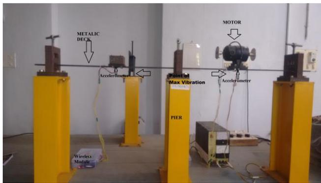
Fig. 9. Field Test 1: Proposed system is tested on a model of a bridge, vibrations are provided on the model using a motor, the amount of vibration produced by the motor is controlled by a voltage source
