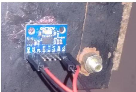
Fig. 10. MEMS Accelerometer fixed using beewax gum on the model of bridge at the point of maximum vibration
