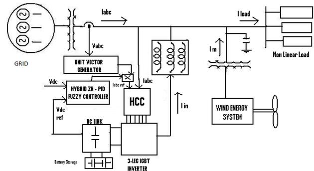
Fig. 2. Inverter interface with combination of battery storage with WEGS
