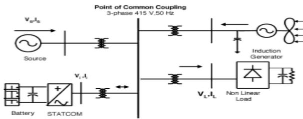
Fig. 1. Schematic diagram of micro-wind generator with battery storage for critical load application.
