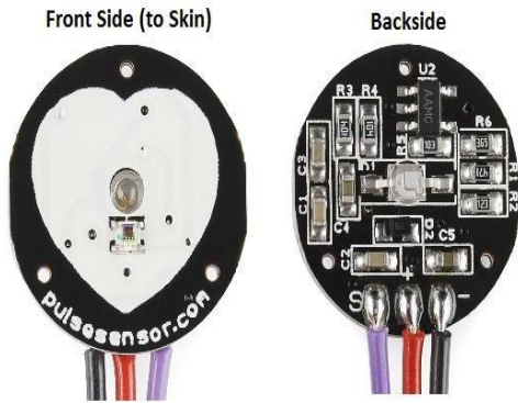
Figure (3) Front & Back view of pulse sensor
