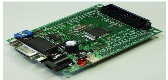
Figure 2 : ARM Microcontroller Board LPC2148
