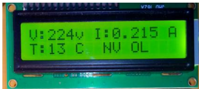
Fig 5.2.1 Load ON Condition
