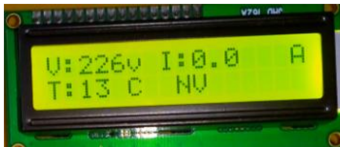
Fig 5.2.2 Load OFF Condition
