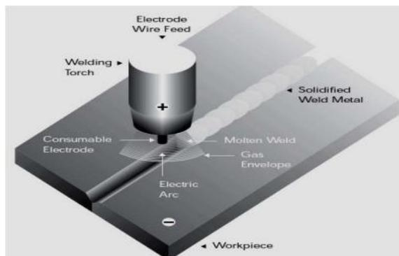
Figure 1: working condition of Work piece
