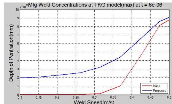
Figure 3: MIG weld concentration at TKG model (max) at t=6e-06
