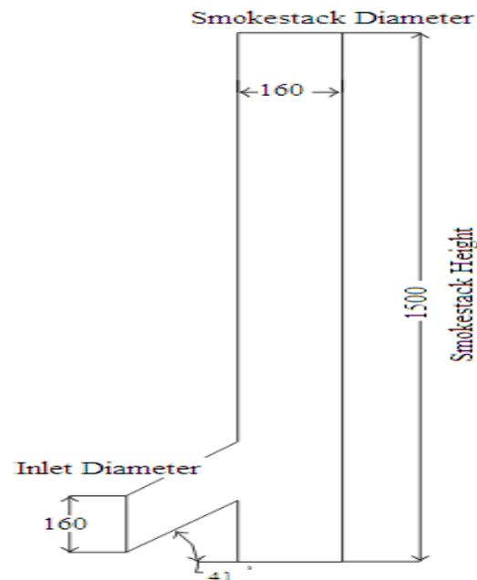
**Figure 7: Smokestack made of GI sheet and its dimensions.**
