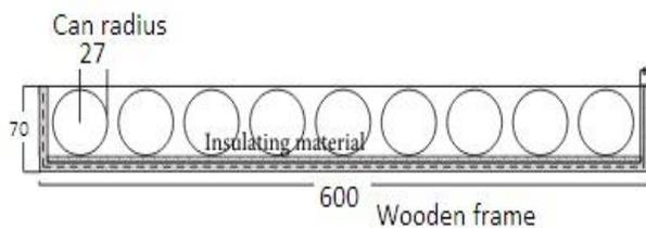
**Figure 5: Photovoltaic collector with 9 columns of recycled aluminum cans (front view).**
