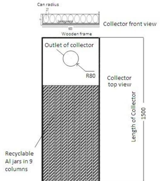
**Figure 6: Photovoltaic collector made of recycled aluminum cans (RAC collector).**
