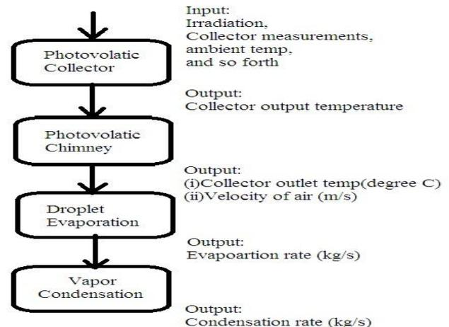
**Figure 4: Flow chart of Photovoltaic desalination system.**
