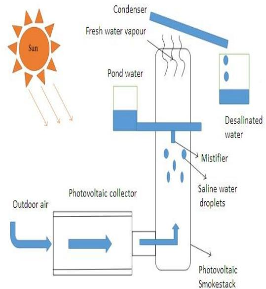
**Figure 3: Schematic diagram of Photovoltaic desalination system.**
