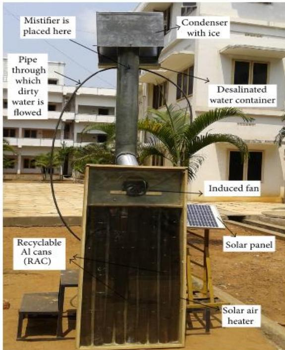
**Figure 8: Desalination plant using a Photovoltaic smokestack with RAC collector.**
