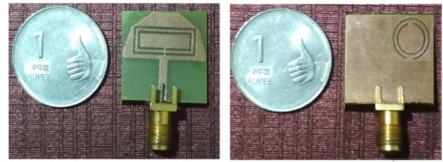
Fig. 3 Photographs of top and bottom view of the fabricated proposed antenna
