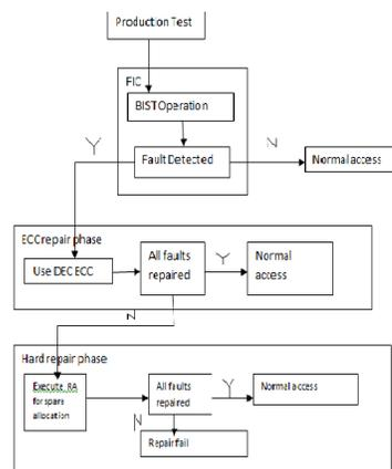
**Fig 1.2 Test and repair flow of Production stage using DEC ECC**
