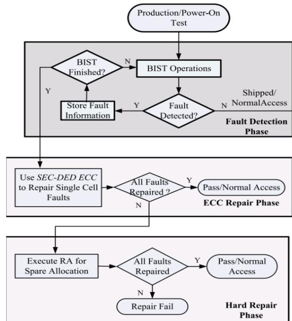
**Fig 1.1 Test and repair flow of the production stage using SEC-DED ECC**
