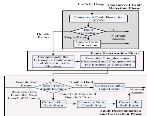
Fig 2 Test and repair flow of Field and Repair stage.
