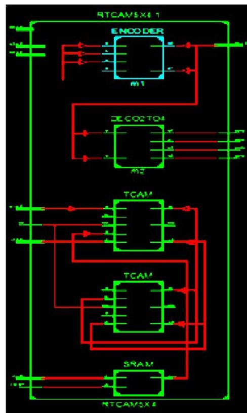
Fig.8. RTL Schematic for Reversible Ternary CAM Using Reversible SRAM and Combinational Logic
