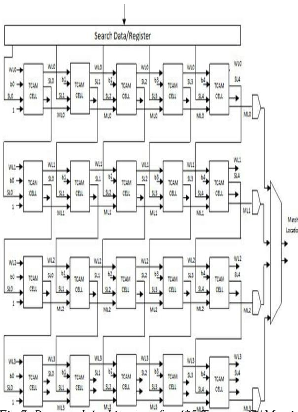
Fig.7. Proposed Architecture for 4\*5 Ternary CAM using Reversible Logic
