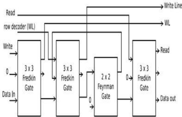
Fig.6. Basic SRAM Cell using Reversible Logic
