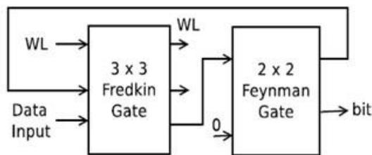
Fig.4. Basic SRAM Cell
