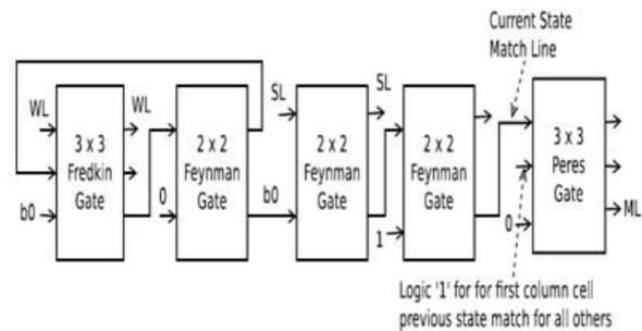
Fig.5. Basic TCAM Cell using Reversible Logic
